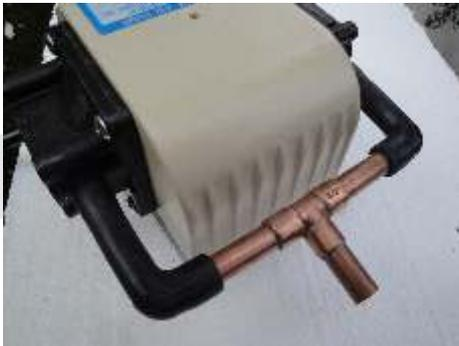
▶ Air pump with replaced manifold, ready to use.
