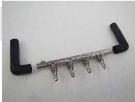
Remove the original manifold from the pump.
