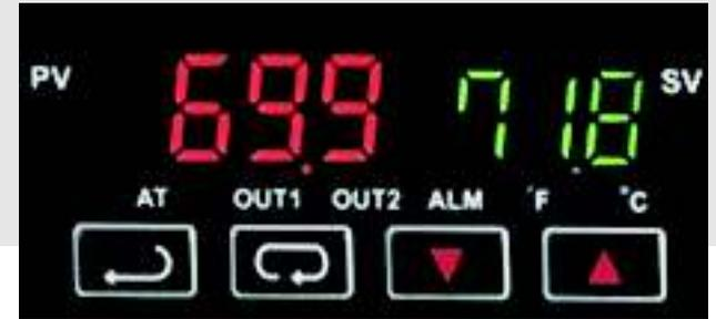
The four buttons below are “Enter”, “Cycle”, “Down”, and “Up”. To set the target humidity, press and hold the up or down arrow until the desired RH is displayed. Then press the enter button to lock the setting in.
