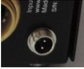
PMCG machines have an alarm connector on the back of the machine. Each machine is shipped with 2 meters of cable and a small red LED light. LED can be located away from the machine, to indicate "RH OUT OF RANGE" status.
