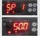
Using up and down arrows, set desired value and press the “P” button. Display change to actual value.
