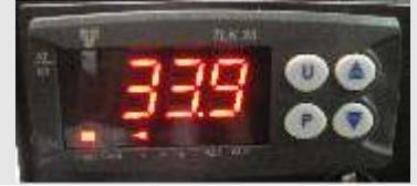
The four buttons on the right are “P-Programm”, “Down”, “Up”, button “U” is not in use. To set the target humidity, press the “P” button, display change to the set mode showing alternately “SP 1” and target value eg. “50.0”.
